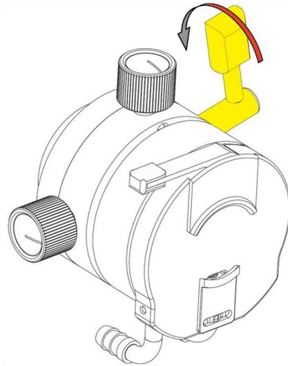
For further specimen orientation, the specimen chuck can also be rotated by 360° as described below:
