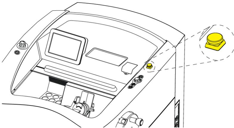
The cutting mode can be changed in three ways. Via the Main screen, in the cutting mode submenu or via the mode button on the right touch panel.
